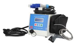
The electrofusion welding unit model Euro MIDI is a polyvalent unit suitable for the welding of all electrofusion fittings up to diameter d. 400. It allows to operator to work at safety voltage lower than 50 Volt, is manufactured according to UNI 10566 and ISO 12176-2 standards, as well as provided with CE mark.
